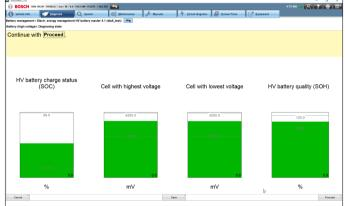
Apart from ESI[tronic] 2.0 Online and a KTS device, no further hardware is required to read out the SOH value. This test step will be offered continuously for additional makes and models wherever supported by the vehicle manufacturer.
